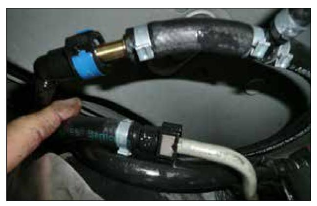
Step 14: Disconnect the factory fuel return line. Using the supplied fuel return hose, attach the male and female quick disconnect fittings to the mating fittings on the factory fuel return line.
