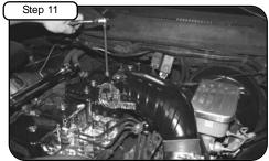
With 6mm hexagonal bit provided and 6mm socket, install the four mounting bolts. Do not tighten completely! Use hex flange head screw provided and install on intake plate. Torque screw to 18 ft. lbs..
