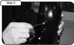
Apply threadlocker to 1/8" NPT plugs. Install to aFe manifold using 3/16" allen key.
