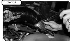
Torque coupler hose clamp with 7/16" deep socket to 71 in. lbs.. Torque the four mounting screws from Step 11 to 18 ft. lbs..
