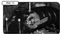
Apply threadlocker to the two 3/8" NPT plugs. Install to top of aFe manifold. Tighten using 5/16" allen key. Torque
