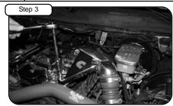
With 10mm socket and extension, remove the 5 screws holding the stock manifold.
