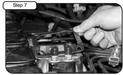
Remove both top and bottom stock gaskets away from air grid heater. Replace with new gaskets provided. (May require a scraper or scotch brite to clean sealing surfaces.)
