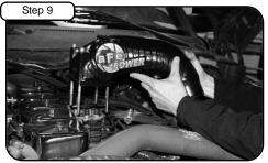
Carefully install aFe manifold into vehicle. Guide screws through gaskets and air grid heater.
