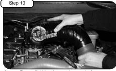
Insert aFe manifold into intercooler coupler hose.
