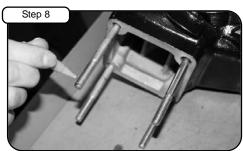
Apply threadlocker to the four mounting screws.
