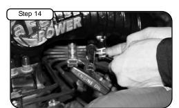
Re-install the engine oil dipstick with socket cap screw provided
