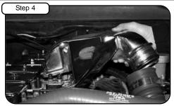
Carefully remove stock manifold out of vehicle. ( Place a clean shop rag over air grid heater to prevent anything
