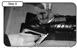
Insert the 2 shorter M8 socket cap screws through aFe manifold. Hold washer against inside mounting flange of aFe manifold and feed screw completely through. Insert the two longer M8 screws w/ washers through the outside mounting bosses
