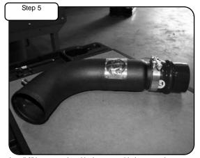
Install 3" hump coupler with clamps provided to new tube.
