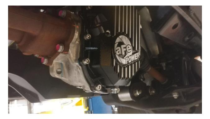
17.Install the supplied M12x1.25 drain plug and crush washer into the bottom of the cover.
