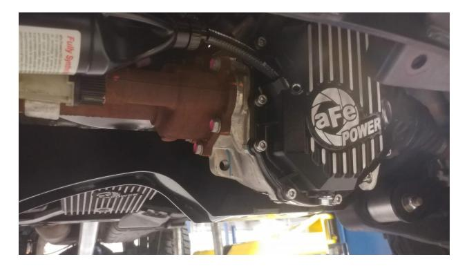
Note: We recommend using a hose or external pump to assist in filling the aFe differential cover.
