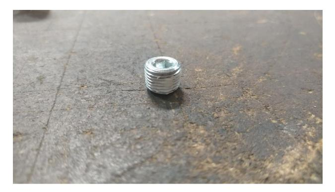
19. Apply Teflon pipe sealant to the threads of the supplied 1/8" NPT plug.
