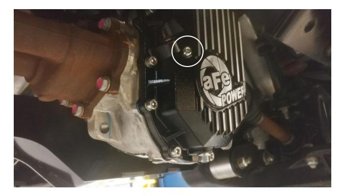
20.Install the 1/8" NPT plug into the side of the cover.
