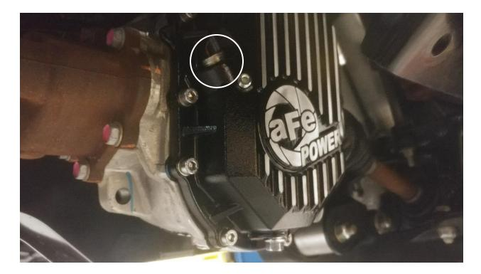
22.Install the 1/2" NPT magnetic 3" deep reach plug into the fill port.
