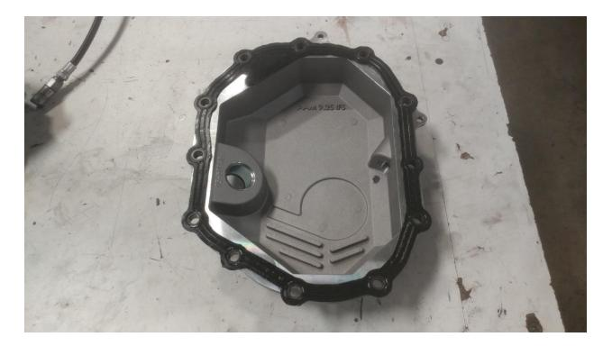
13.Align the OEM gasket and supplied aFe differential cover into position using the correct orientation shown above.
