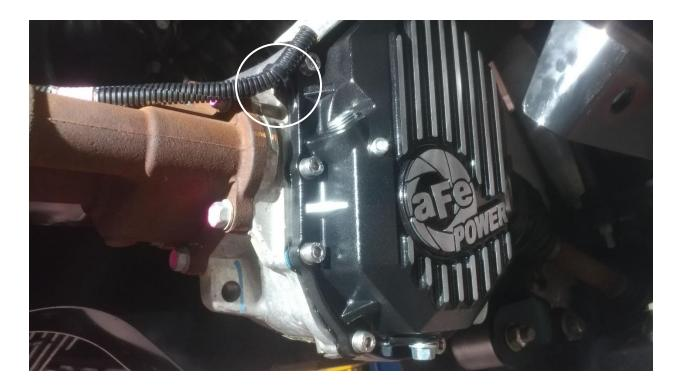
23.Reconnect the four wheel drive actuator wire to the left side and top of the aFe differential cover.
