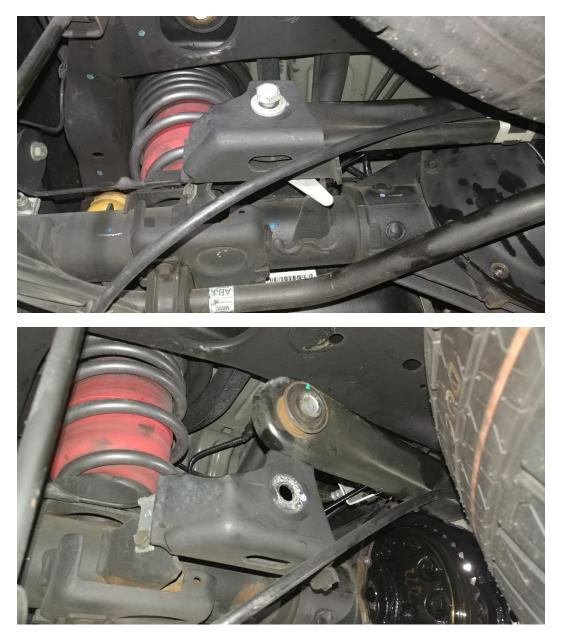
Note: Steps 5-6 are for coil spring vehicles only and must be completed with the vehicle on the ground, in a static position.
