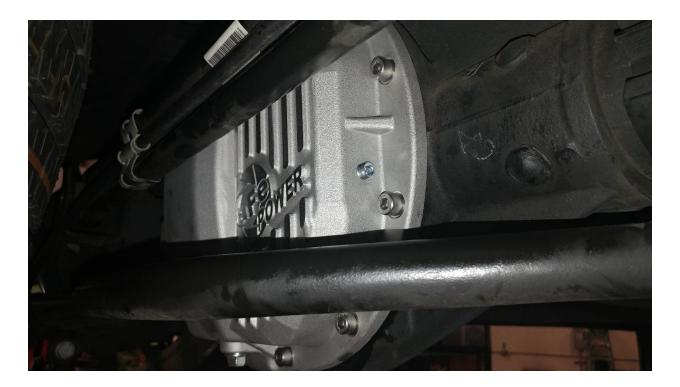
21. Apply Teflon pipe sealant to the threads of the 1/8" NPT plug and install into the side of the cover.
