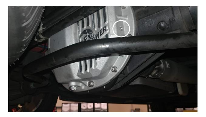
20. Fill the aFe differential cover using new gear oil. Fill until gear oil runs out of the 1/8" NPT port on the side of the cover (about 3 1/2 quarts).
