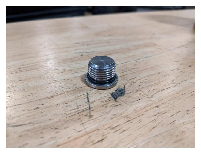
19. Apply gear oil to the provided -016 O-Ring, then install it on the provided M18x1.5 plug.
