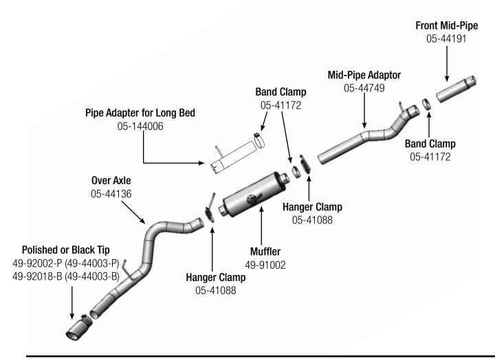
**Step 1: (Read Instructions prior to installation)** Remove your stock exhaust up to the cataytic converter from the rear of your truck working your way forward. It may be necessary to cut the pipes if the slip joints are stuck. Take caution not to damage the factory isolation mounts as they will be reused.
