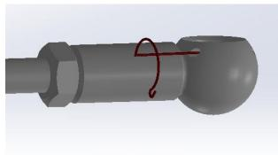
25. Remove the locking wire securing the front exhaust valve linkages to the exhaust valve with a pick or small screwdriver (See Image). Retain for later use.
