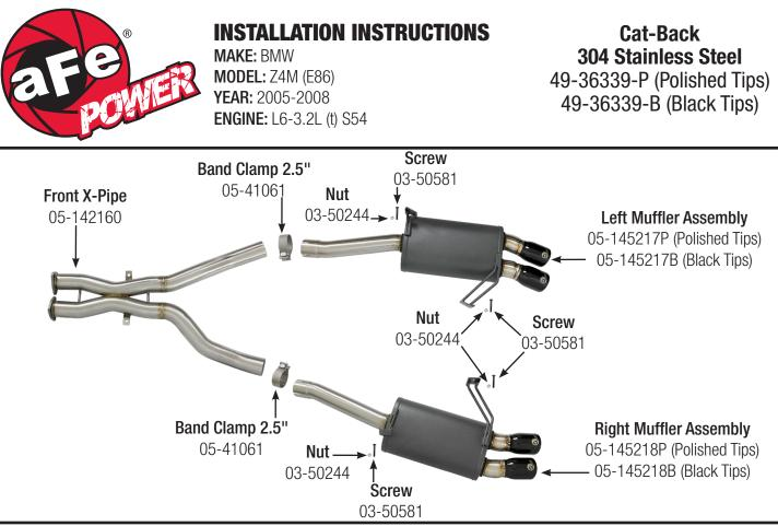
**Caution:** Allow time for your vehicle to cool down prior to installation. When working on or under your vehicle proceed with caution. Exhaust systems reach high temperatures and may cause serious burns. Wear protective safety equipment; eye goggles and gloves to ensure a safe installation. **aFe recommends professional installation on our products.**
