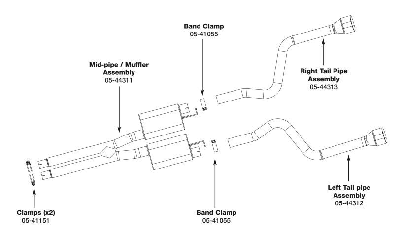
**Step 1:** (Read Instructions prior to installation) Remove your stock exhaust from the rear of your truck working your way forward. Disconnect the ground strap from chassis to muffler and save for re-use later. Also take caution not to damage the factory isolation mounts as they will be reused. It is recommended to not fully tighten the clamps until the entire system has been installed.
