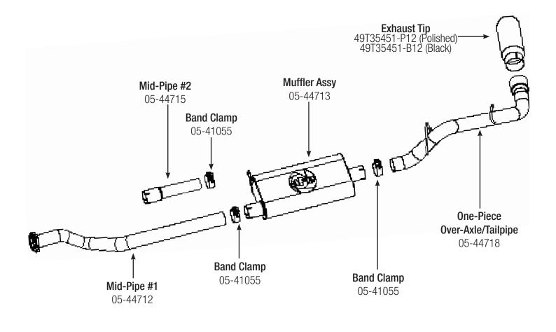
**Step 1: (Read Instructions prior to installation)** Remove your stock exhaust up to the catalytic converter from the rear of your truck working your way forward. Take caution not to damage the factory hardware and isolation mounts as they will be reused.
