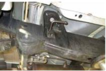
NOTES: aFe recommends that the tailpipe be at least 1/2"-1" away from any body panels to avoid heat related body damage. Tighten and secure.
