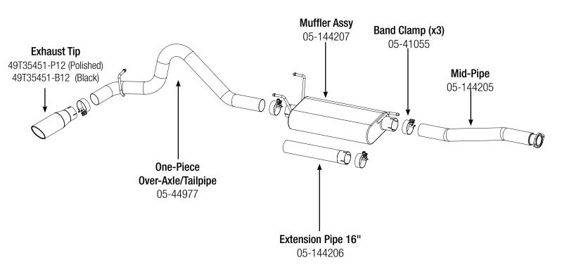
**Step 1: (Read Instructions prior to installation)** Remove your stock exhaust up to the catalytic converter from the rear of your truck working your way forward. Take caution not to damage the factory hardware and isolation mounts as they will be reused.
