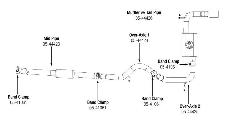
**Step 1: (Read Instructions prior to installation)** Remove your stock exhaust from the rear of your truck working your way forward. Take caution not to damage the factory isolation mounts as they will be reused. It may be helpful to lubricate the isolation mounts prior to disassembly. It is recommended to not fully tighten the clamps until the entire system has been installed.
