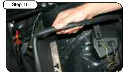
Install trim seal on housing and drop housing into vehicle. Do not tighten down housing.
