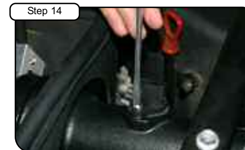
Install MAF sensor onto tube using provided gaskets, spacers and screws.
