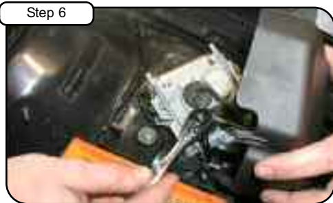
Remove plastic cover from headlight controller via locking tabs. Using a 10mm socket, remove the (2) bolts securing controller to allow for its movement and to release lower half of airbox.
