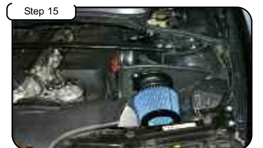
Place enclosed CARB EO sticker on a clean/smooth surface on or near device. EO identification label is required in passing the Smog Check Inspection. Make sure all hoses and clamps are tight and that all electrical components (if applicable) are secure. Check and retighten connections and filter after a few hours of operation.
