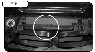
Grill suppot should pass throught the clearance hole in the DAS.
