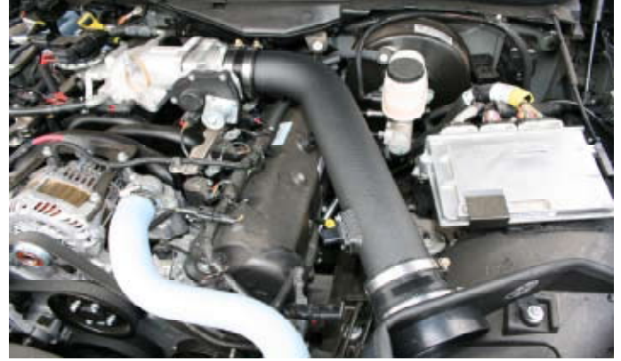
15- Place the coupling with clamps onto the adapter and slip the intake tube into position like shown.
