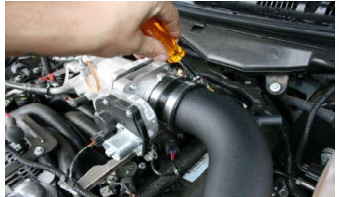
16- When the tube is in position, tighten all four clamps on the couplings securing it to the vehicle.
