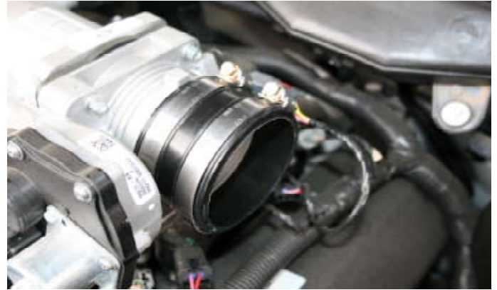
14- Place the straight coupling onto the throttle body with the clamps in position.
