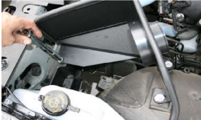
11- Place housing into vehicle and re-use the existing nuts and mounting locations.
