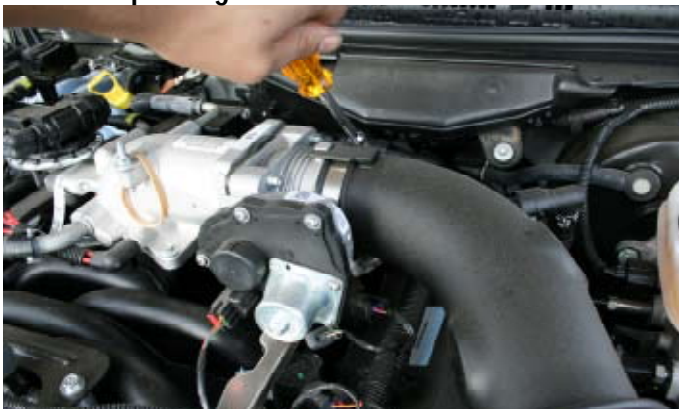
3- Loosen the clamp at the throttle body
