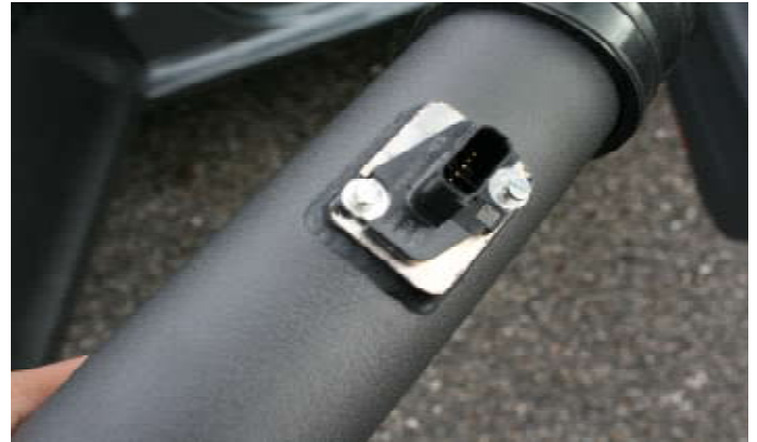
13- Install the MAF sensor into your aFe intake tube using the supplied bolts.
