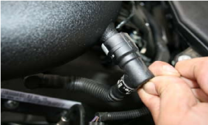
17- Plug the crank case vent line onto your new aFe intake tube.
