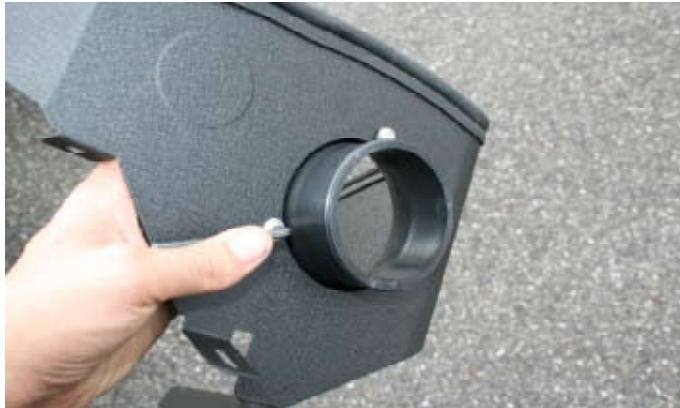
10- Using a 4mm allen key, install the adapter using the three supplied screws and washers.
