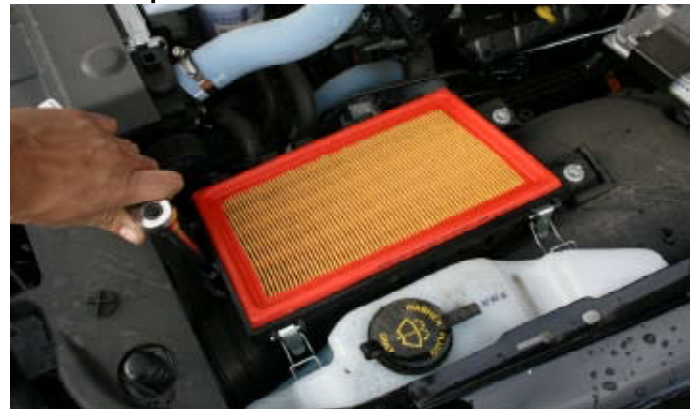
7- Using a ratchet with extension, Remove the lower intake boxes three mounting bolts.
