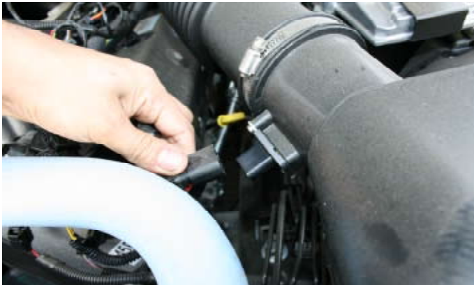
2- Disconnect the MAF sensor by pulling out the red safety lock and squeezing.
