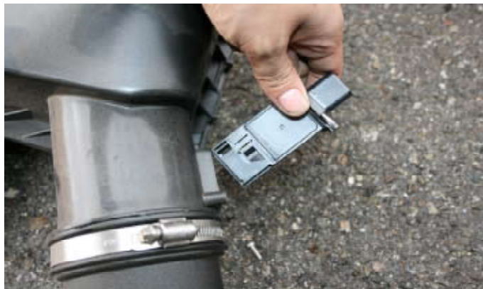
12- Unscrew the MAF sensor from the stock air intake box and remove.
