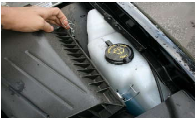
4- Disconnect the two pressure clips on the intake box housing.
