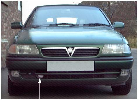
Feed the flexi cold air hose down to the front lower grille. Attach the hose to the grille using the long plastic tie supplied.
