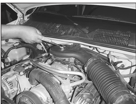
2. Loosen the nut at the intake plenum as shown.
