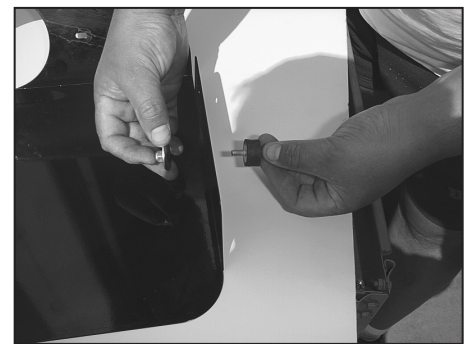
8. Install the two rubber isolator stand off's using the provided hardware as shown.
