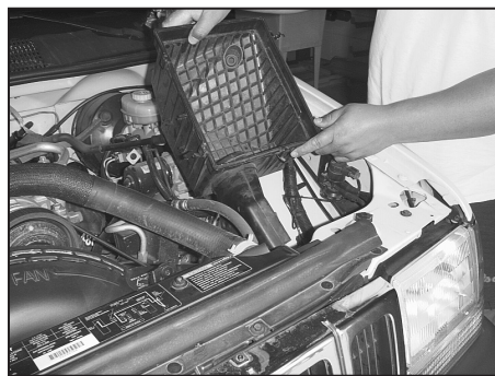
6. Remove the air box base as shown. NOTE: K&N Engineering, Inc., recommends that customers do not discard factory air intake.
