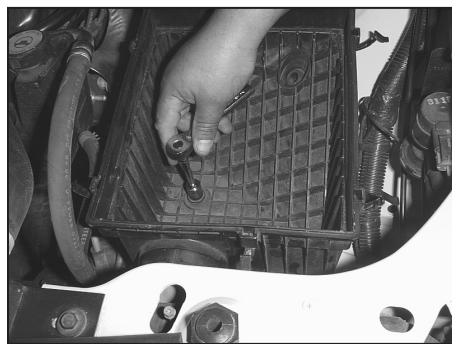
5. Using a 1/2" socket, loosen and remove the three bolts that secure the air box base.
