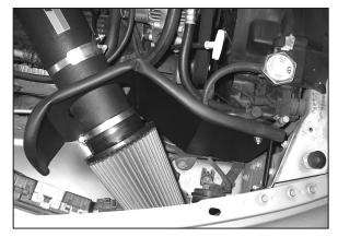
26. Install the  $K\&N^{\otimes}$  air filter element onto the intake tube and secure with hose clamp.
