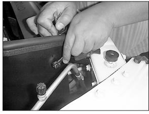
15a. Dakota models only, mount the heat shield to the short "C" bracket (070672) using the lower hole on the heat shield.
