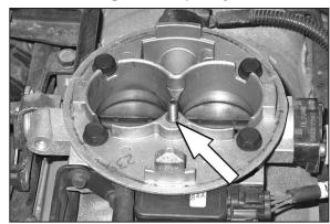
20. Install the set screw into the threaded hole in the throttle body and tighten.
