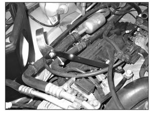
19. Install the saddle bracket assembly using the bolt removed in previous step.
