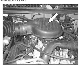
2. Loosen and remove the nut at the intake plenum as shown.
