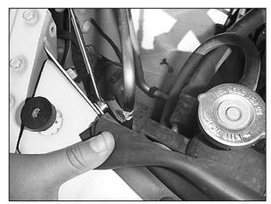
11. Dakota models only, loosen and remove the core support bolt.
