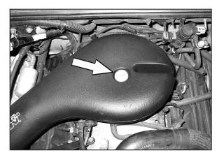
23. Install the intake tube onto the throttle body and secure the plenum with the provided nut extension, and washer.
