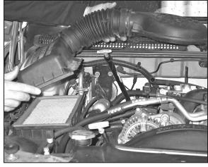
5. Remove the intake plenum and airbox.
