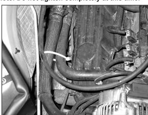
16. Using one of the provided zip ties, secure the A/C line and heater hose together as shown. Note: when installing the K&N® intake tube, check the two hoses for clearance under the intake tube and adjust for best fit.
