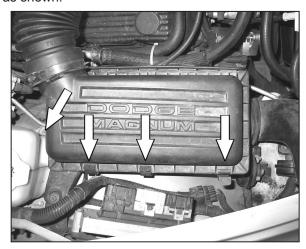
3. Using a flat blade screwdriver, detach the (4) airbox clips.
