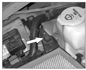
6. Loosen and remove the nut that secures the airbox base.
