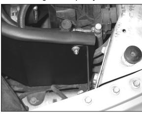
15b. Durango models only, mount the heat shield to the long "C" bracket (070682) using the upper hole in the heat shield.
