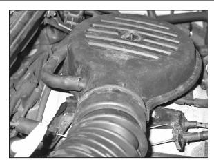
4. Remove the crankcase vent hose from intake plenum.
