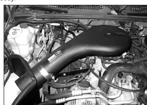
22. Slide the intake tube through the hole in the heat shield as shown.
