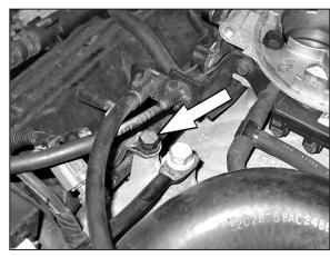
18. Loosen and remove the bolt that retains the fuel rail bracket.
