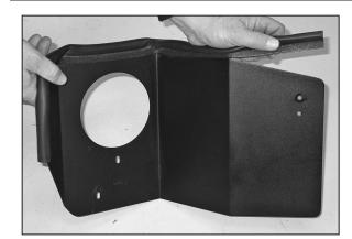
10. Install the trim seal onto the heat shield.
