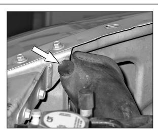
7. Using a flatblade screwdriver, pry the push clip on the air inlet duct.
