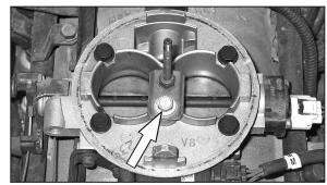
9. Loosen and remove the bolt that secures the stud assembly. Remove the stud assembly and OE gasket.
