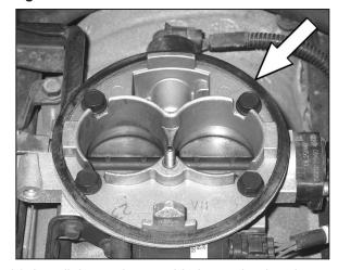
21. Install the gasket provided onto the throttle body.
