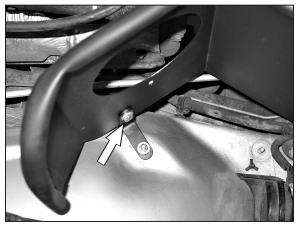
14. Mount the heat shield to the long "L" bracket (070662).
