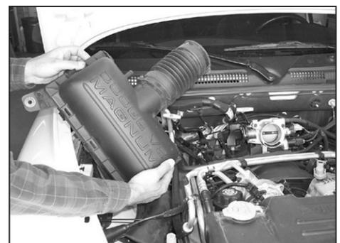
7. Pull firmly upwards on the stock air box to remove from the vehicle as shown.
