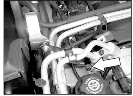
20. Install the saddle bracket assembly onto the A/C compressor with the bolt that was removed in step 19.
