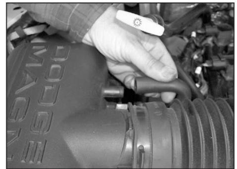
5. Remove the vent hose from the air box as shown.
