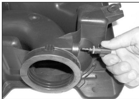
3b. To remove temperature sensor from resonator, turn sensor 1/8 of a turn counter clockwise and remove the sensor as shown.
