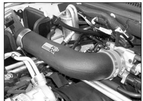
22. Install the intake tube onto the throttle body as shown.
