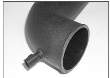
21c. Remove the factory O-ring from the temperature sensor, then install the sensor into the intake tube as shown.
