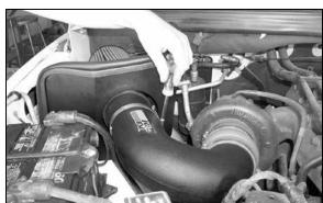
19. Attach saddle bracket to the intake tube with hose clamp provided. Adjust the bracket to achieve appropriate clearance for intake tube and tighten hardware.
