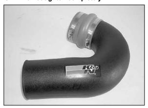
9. Attach the hump hose onto the  $K\&N^{\otimes}$  intake tube as shown.
