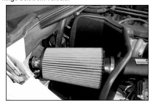
16. Install the air filter onto the intake tube. NOTE: Do not tighten completely.
