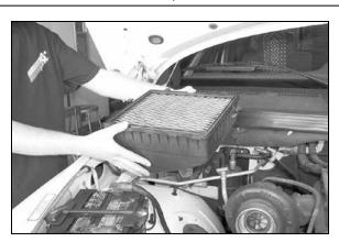
4. Pull upward firmly on the airbox base to release it from it's mounting studs and remove.
