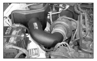
11. Slide the K&N® intake tube through the heat shield and attach the hump hose to the flange on the turbo.
