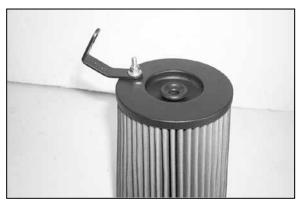
12. Install filter bracket provided onto the stud on the top plate of the air filtert as shown. NOTE: Do not tighten completely.
