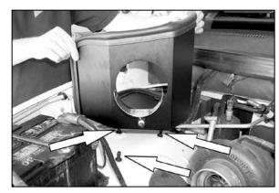
Install heat shield onto the locating studs as shown above.
