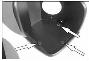
6. Install the three grommets provided onto the heat shield as shown.
