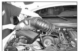
3. Release the 4 clips that retain the airbox top to the airbox base. Detach the intake tube from the flange on the turbo and remove the upper air intake assembly.
