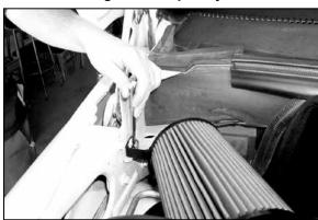
17. Attach the filter bracket to inner fender using the bolt removed in step 15.
