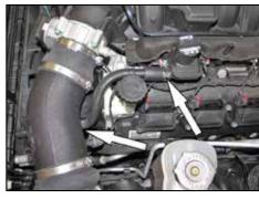
21. Install the assembled vent hose onto the fitting installed in the K&N® intake tube and then attach the open end to the valve cover port and secure with the provided hose clamp.
