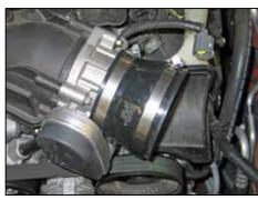
14. Install the silicone step hose (08497) onto the throttle body and secure with the provided hose clamp.
