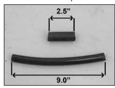
19. Cut the provided  $\frac{1}{2}$ " silicone vent hose to a length of 9" long, and cut the  $\frac{5}{8}$ " vent line to a length of 2.5" long.
