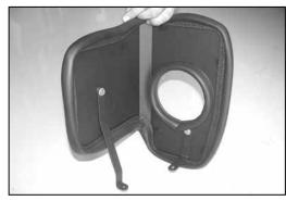
28. Install the two brackets onto the heat shield with the provided hardware as shown. Do not tighten completely.
