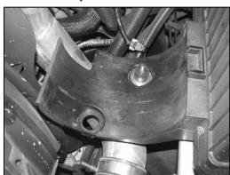
11. Install the rubber mounted stud onto the air box mounting bracket with the provided hardware as shown
