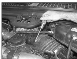
5. On vehicles equipped with a two piece inlet tube and bellows, loosen the hose clamp that secures the turbo inlet tube to the inlet bellows.
