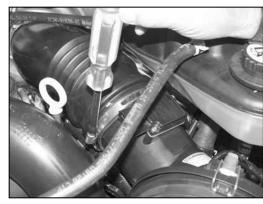
5a. On vehicles equipped with a one piece inlet tube and bellows, loosen the hose clamp securing the inlet tube and bellows to the air box assembly.
