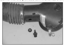
18a. On vehicles equipped with an air temperature sensor, remove the air temperature sensor and grommet as shown.
