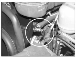
25a. On vehicles equipped with an air temperature sensor, reconnect the air temperature sensor electrical connection as shown.
