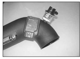
21. On vehicles equipped with a mass air sensor, install the mass air sensor into the K&N<sup>®</sup> intake tube with the provided screws and spacers as shown.
