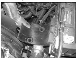
10. Remove the rubber grommets that retain the air box assembly onto the vehicle.
