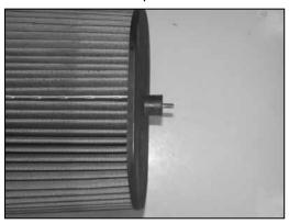
31. Install the provided rubber mounted stud onto the K&N® air filter as shown.
