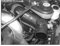
22. Install the  $K\&N^{\otimes}$  intake tube onto the turbo inlet with the provided hose clamp.
