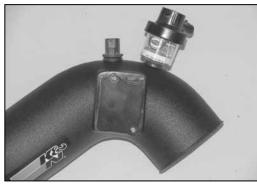
21d. On vehicles equipped with an air temperature sensor, install the factory grommet and air temperature sensor into the hole that was drilled in the previous step.
