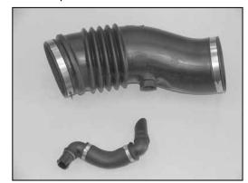
15b. On vehicles equipped with a one piece inlet tube and bellows, cut the band clamp that secures the crank case vent tube to the turbo inlet tube. Then remove the crank case tube assembly from the turbo inlet tube as shown.
