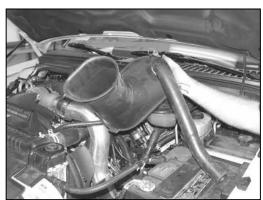
9. Remove the air box top as shown.
