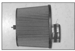
31a. Install the provided silicone hose (08761) onto the air filter flange and secure with the provided hose clamp.
