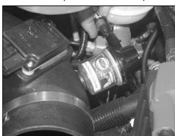
24. Reconnect the restrictor gauge electrical connection as shown.
