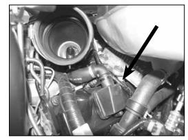
9b. On vehicles equipped with a one piece inlet tube and bellows, using a large screwdriver, pry up on the crank case vent fitting in the valve cover to disengage it from the valve cover.
