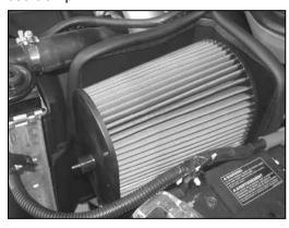
32. Install the air filter element onto the intake tube as shown.
