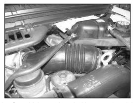
9a. On vehicles equipped with a one piece inlet tube and bellows, loosen the hose clamp that secures the inlet tube and bellows assembly to the turbo inlet.
