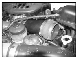
15. On vehicles equipped with a two piece inlet tube and bellows, install the silicone hump hose (08418) onto the stock turbo inlet tube and secure with the provided hose clamp as shown.
