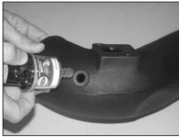
17. Install the factory grommet and restriction gauge into the K&N® intake tube as shown.
