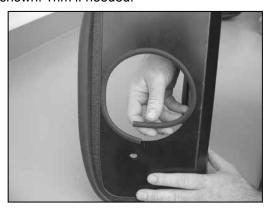
27. Install the edge trim onto the inner hole on the heat shield as shown. Trim if needed.
