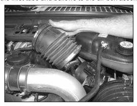
6. On vehicles equipped with a two piece inlet tube and bellows, loosen the hose clamp at the mass air sensor and remove the intake hose from the vehicle.
