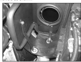
30. Mount the heat shield onto the rubber mounted stud and then secure the long "L" bracket onto the air box mount with the provided bolt and washers.
