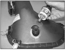
16. Remove the air filter restriction gauge and grommet from the factory air box.
