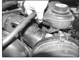
3a. On vehicles equipped with an air temperature sensor, disconnect the air temperature sensor electrical connection as shown.
