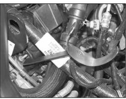
14. Install the saddle bracket assembly onto the engine block and secure with the nut removed in step 12.
