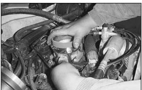
28. Install the silicone hose over the throttle body adapter and tighten using a provided midi hose clamp.
