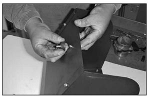
20. Using the provided hardware, install the rubber mounted studs onto the bottom side of the heat shield.
