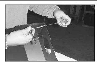
18. Using a 1/8" allen wrench and a 3/8" socket, assemble the heat shield using the provided hardware.
