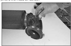
13. Remove the air temperature sensor from the factory intake tube.
