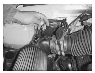
5. Disconnect the air temperature sensor electrical connection.
