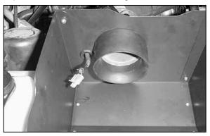
25. Install the factory air temperature sensor lead through the grommet hole on the heat shield.
