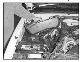
8. Remove the lower airbox assembly.
