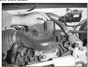
2. Loosen and remove the tall wing nut on the throttle body.
