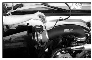
30. Fully install the K&N® intake tube onto the throttle body adapter and tighten second midi hose clamp.
