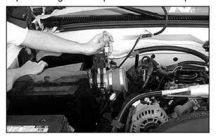
27. Install the mass air adapter onto the mass air sensor and tighten mass air sensor side only.
