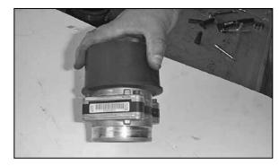
21. Install the filter adapter onto the mass air sensor with the directional arrow as shown above.
