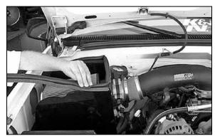
32. Install trim seal onto the heat shield. NOTE: Some cutting and trimming may be necessary to achieve best fit.
