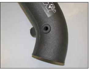
15. Install the provided rubber grommet into the  $K\&N^{\circledast}$  intake tube as shown.
