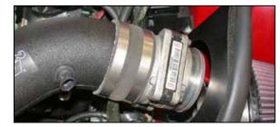
28. Install the mass air sensor assembly onto the  $K\&N^{\otimes}$  intake tube and secure with the provided hose clamp.
