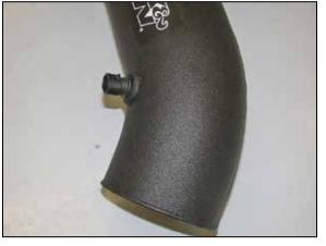
16. Install the air temperature sensor from step #14 into the grommet in the K&N<sup>®</sup> intake tube as shown.
