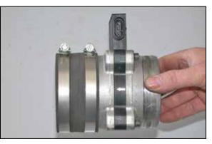
27. Install the silicone hose (#08630) onto the intake tube side of the mass air sensor and secure with the provided hose clamp.
