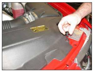
2. Release the center pin on the five radiator cover clips. Then remove the clips from the radiator cover.
