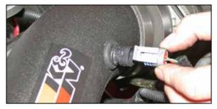
31. Reconnect the temperature sensor electrical connection.
