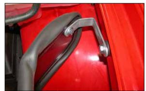
25. Install the heatshield bracket (#010062) onto the heatshield and inner fender and secure with the provided hardware.
