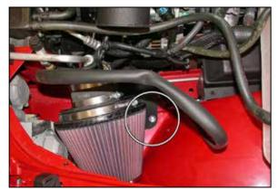
23. Secure the heatshield to the inner fender with the 6mm bolt provided. NOTE: Thread the 6mm bolt into the hole vacated in step #11.
