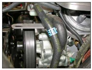
12. Install the tube bracket #010061 using the provided hardware.
