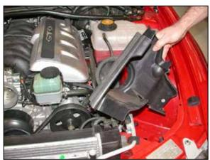
10. Lift up and pull out the air deflector from behind the head light
