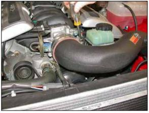
17. Install the K&N<sup>®</sup> intake tube onto the throttle body as shown and secure with the provided hose clamp, using the 8mm bolt provided. Secure the K&N<sup>®</sup> intake tube onto the mounting bracket installed in step #12.
