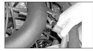
28. On vehicles equipped with air injection pump, attach the air injection hose to the fitting on the K&N® intake tube.
