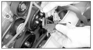
11. On vehicles equipped with air injection pump, detach the vacuum hose from the air control solenoid valve vacuum control solenoid valve.
