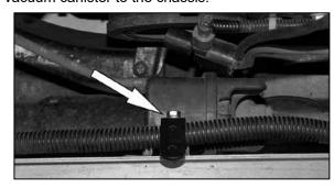
17b. Using the provided hardware, install the provided bracket (083155) along with the provided spacer and the factory vacuum canister.
