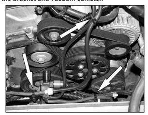
17c. Using the provided hardware, secure the vacuum solenoid to the lower hole in the bracket. Then secure the vacuum line to the upper hole with the provided mounting head tie wrap. Using the two remaining tie wraps, secure the vacuum lines to the wiring harness.
