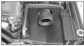
32. Install the radiused adapter onto the  $K\&N^{\otimes}$  intake tube.
