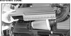
2. Release the 6 clips that retain the air box top, then remove the top.
