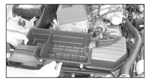
7. Loosen and remove the 3 bolts that secure the air cleaner base, then remove the air cleaner base. NOTE: K&N Engineering, Inc., recommends that customers do not discard factory air intake.
