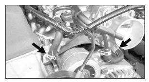
9. Detach the coolant hose from the fitting on the intake manifold, and from the fitting on the underside of the throttle body.
