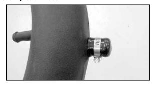
28a. On vehicles not equipped with an air injectino pump, install the provided "Caplug" onto the vent port on the K&N® intake tube and secure with the provided hose clamp as shown.
