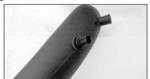
26c. Remove the air temperature sensor from the stock intake tube and install it into the grommet installed in the K&N® intake tube in the provious step as shown.
