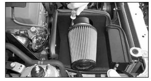
33. Install the K&N® air filter onto the K&N® intake tube and secure with the provided hose clamp. NOTE: Drycharger® air filter wrap; part number RC-5149DK is available to purchase separately. To learn more about Drycharger® filter wraps or look up color availability please visit http://www.knfilters.com®.
