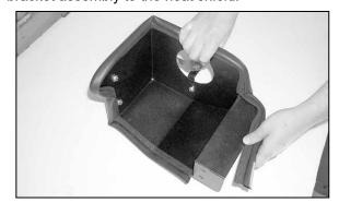
22. Install the edge trim to the heat shield assembly.
