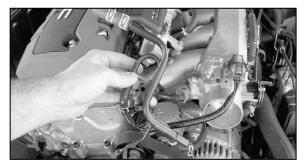
13. Remove the pipe assembly.
