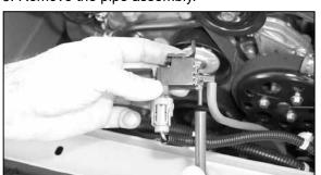
14. On vehicles equipped with air injection pump, attach the provided 4mm (long) vacuum hose to the air control solenoid valve.
