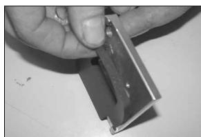
20. Apply the provided gasket to the mass air sensor adapter as shown; sticky side down.
