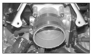
18. Install the provided silicone hose (08690) onto the throttle body with the provided hose clamps as shown.
