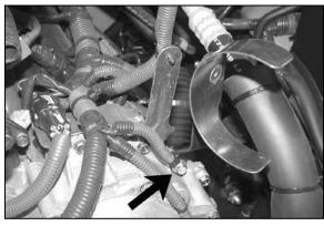
17. Install the saddle bracket assembly and ground wire removed in step #16 with the provided hardware as shown.
