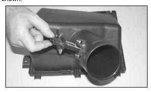
19. Remove the two screws that secure the mass air sensor to the air box lid, then remove the mass air sensor as shown.
