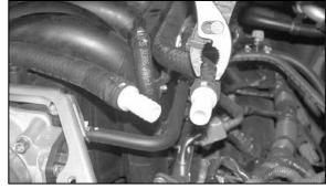
26. Install the provided hose mender into the two crank case vent hoses and secure the existing spring clamps as shown.
