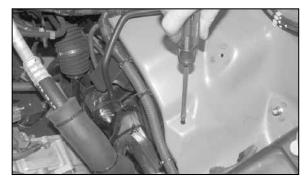
13. Using a screw driver, push the center of the plastic inner fender retaining clip through, then remove the clip from the inner fender.
