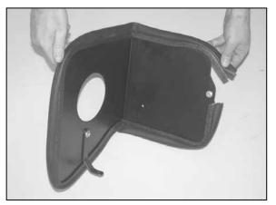
12. Install the edge trim onto the heat shield as shown. Trim as needed.
