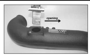
22. Install the mass air sensor assembly into the intake tube with the opening of the sensor pointing towards the air filter end of the tube as shown.
