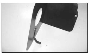
11. Install "L" bracket (07190) onto the heat shield as shown.
