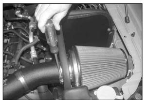
30. Install the K&N<sup>®</sup> air filter assembly onto the K&N<sup>®</sup> intake tube as shown; secure with the provided hose clamp.
