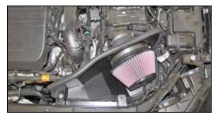
15. Set the heat shield assembly into the vehicle. The mounting stud will insert into the factory air box mounting grommet and the front of the heat shield will be secured to the core support with the provided hardware.
