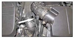
3. Disconnect the crank case vent hose from the factory intake tube.
