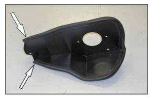
9. Install the provided edge trim around the heat shield as shown.
