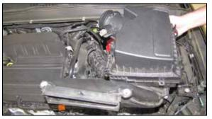
6. Lift up the air box to dislodge it from the mounting grommets and then remove it from the vehicle.
