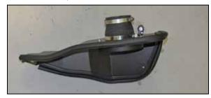
13. Install the provided step coupler (084055) onto the filter adapter and secure with the provided hose clamp.
