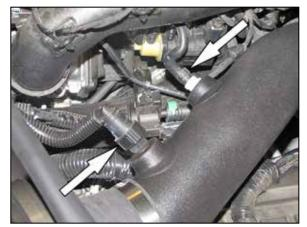
22. Connect the factory solenoid vent hose and the factory crank case vent hose to the fittings installed into the K&N<sup>®</sup> intake tube.
