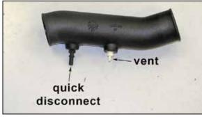
17. Install the provided 1/4 npt fittings into the K&N<sup>®</sup> intake tube as shown.
