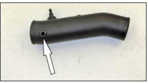
18. Install the provided inlet air temperature sensor grommet into the K&N<sup>®</sup> intake tube.
