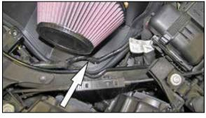
16. Clip the inlet air temperature sensor harness into the hole provided in the heat shield.
