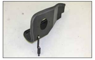
11. Install the mounting bracket assembly onto the heat shield as shown using the provided hardware.
