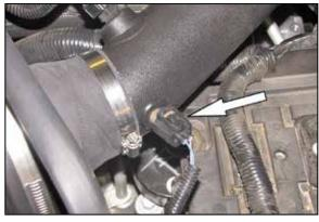
23. Connect the inlet air temperature sensor electrical connection.
