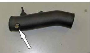
20. Install the inlet air temperature sensor into the grommet installed into the K&N<sup>®</sup> intake tube.
