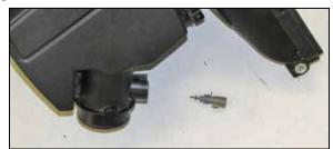
19. Remove the inlet air temperature sensor from the factory air box and remove the O-Ring from the sensor.
