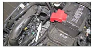
8. Install the provided hump hose (087121) onto the turbo inlet and secure with the provided hose clamp.
