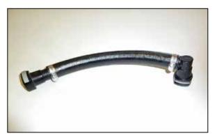
16A. On some later models it may be necessary to assemble the crank case vent hose assembly with the provided parts and install due to the manufacturer changing the position on the valve cover port. Install the assembly with the 90° fitting attached to the valve cover port.
