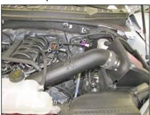
Install the K&N<sup>®</sup> intake tube into the coupling hose at the filter adapter and then into the hose at the throttle body, adjust the tube for best fit and then secure with the provided hose clamps.
