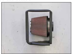
9. Install the K&N<sup>®</sup> air filter onto the filter adapter and secure with the provided hose clamp. NOTE: Drycharger® air filter wrap; part # RC-5173DK is available to purchase separately. To learn more about Drycharger® filter wraps or look up color availability please visit http://www.knfilters.com®.
