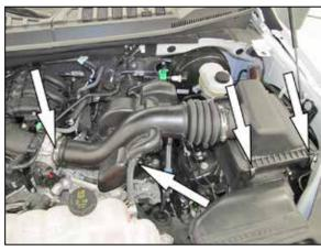
4. Loosen the hose clamp securing the intake tube to the throttle body, unhook the coolant reservoir hose from the intake tube and unclip the two upper air filter housing retaining clips. Then remove the upper air filter housing and intake tube assembly.
