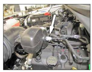
3. Disconnect the EVAP vent quick connect fitting.
