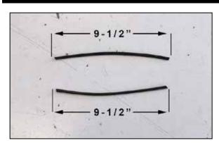
7. Cut the provided small edge trim into two lengths of 9-1/2" as shown.
