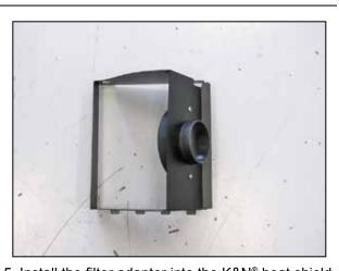
5. Install the filter adapter into the K&N $^{\! \otimes}$  heat shield as shown and secure with the provided hardware.
