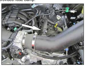
15. Connect the crank case vent guick disconnect fitting to the mating quick disconnect fitting installed into the K&N® intake tube.
