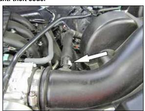
2. Disconnect the Crank case vent hose quick connect fitting.
