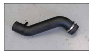
12. Install the provided hump coupler hose (08699) onto the K&N® intake tube and secure with he provided hose clamp
