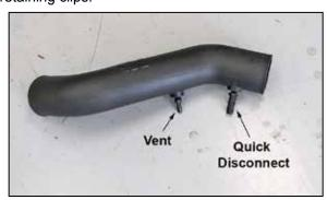
11. Install the provided NPT quick disconnect fitting and NPT vent fitting into the K&N® intake tube as shown.
