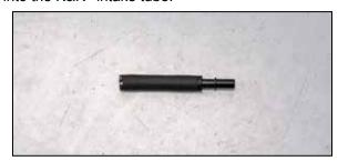
16. Install the provided EVAP vent hose onto the provided quick disconnect union as shown.
