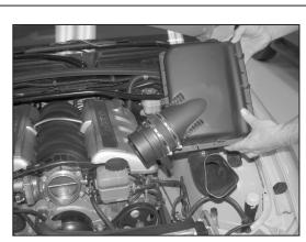
7. Pull up on the air box assembly to dislodge it from the three mounting pins and then remove the air box from the vehicle as shown.
