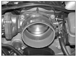
16. Install the silicone hose (08625) onto the throttle body and secure with the provided hose clamps as shown.
