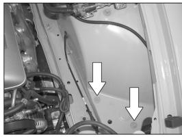
8. Remove the three air box mounting pins shown with a T-30 torx socket.
