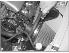
13. Install the heat shield assembly onto the inner fender and start the mount bolts in the air box mounting pin holes, then place the K&N® air filter into position. Tighten the heat shield mounting bolts, then install the K&N® air filter onto the filter adapter and secure with the provided hose clamp.
