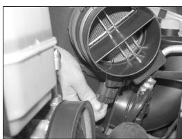
6. Release the mass air sensor electrical connection clip, then disconnect the electrical connection.
