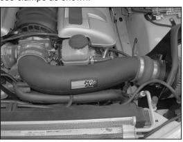
18. Install the K&N® intake tube into the silicone hose attached to the throttle body and then onto the mass air sensor. Secure with the provided hose clamps as shown.
