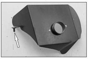
6. Install one of the provided mounting studs onto the heat shield and secure with the provided hardware.
