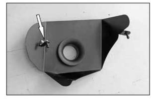
7. Install the remaining mounting stud onto the long leg of the provided "L" bracket (064340) and secure with the provided hardware, then install the assembly onto the heat shield as shown using the provided hardware.
