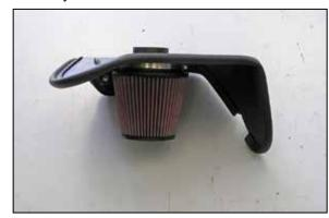
9. Install the K&N<sup>®</sup> air filter onto the filter adapter and secure with the provided hose clamp.
