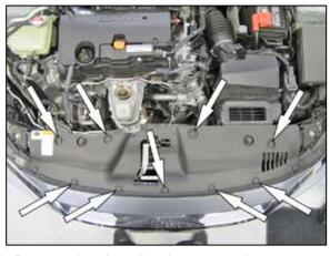
2. Remove the nine clips that secure the core support cover and then remove the cover from the vehicle.
