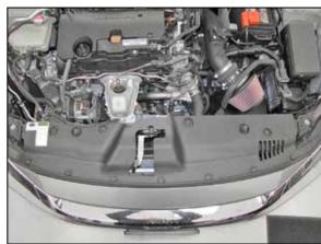
22. Reinstall the core support cover and secure with the factory retaining clips.
