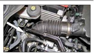
5. Loosen the two hose clamps that secure the intake tube to the air filter housing and the throttle body, Loosen the spring clamp securing the crank case vent hose and then remove the intake hose from the vehicle.
