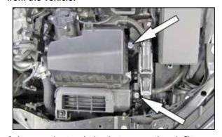
6. Loosen the two bolts that secure the air filter housing, apply some spray lubricant to the mounting grommet and then remove the air filter housing from the vehicle.
