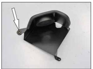
10. Remove the mounting grommet from the factory air filter housing and install it into the K&N® heat shield as shown.
