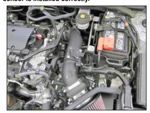
19. Install the K&N® intake tube into the coupling hoses, adjust for best fit and then secure with the provided hose clamps.
