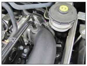
20. Install the crank case vent tube into the grommet installed into the K&N® intake tube.
