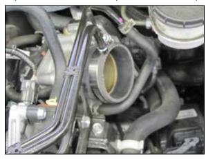
14. Install the coupling hose (08284) onto the throttle body and secure with the provided hose clamp.
