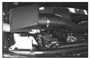
6. Release the four upper air box clam shell clamps, then remove the upper air box and intake tube assembly.
