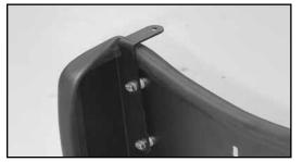
9. Install the small "L" bracket (#070742) onto the inner fender, behind the hood support. Secure with the provided hardware as shown.
