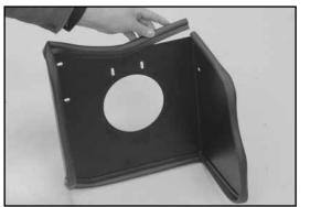
10. Install the long edge trim onto the heat shield as shown.
