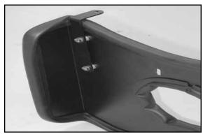
12. Install the long "L" bracket (#070902) onto the heat shield with the provided hardware as shown. Note: Place two of the provided spacers between the bracket and heat shield, one on each bolt.
