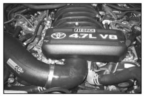
34. Re-install the engine cover and secure with the factory nuts.
