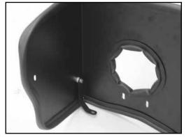
13. Install the provided "C" bracket onto the heat shield with the provided hardware as shown. Note: One provided spacer is to be placed between the bracket and heat shield.
