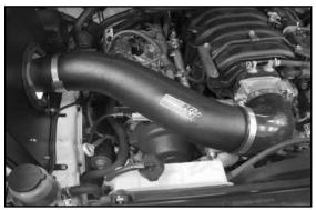
27. Install the K&N<sup>®</sup> intake tube into the silicone
