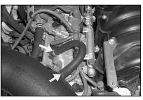
28. Install the provided crank case vent hose onto the valve cover fitting, then connect the open end to the NPT fitting installed into the K&N® intake tube as shown.
