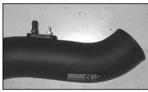
26. Install the provided 1/4" NPT fittings into the K&N<sup>®</sup> intake tube as shown.
