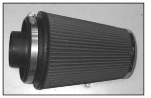
30. Install the provided air filter adapter into the K&N<sup>®</sup> air filter and secure with the provided hose clamp as shown.
