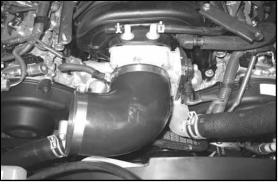
21. Install silicone hose (#084086) onto the throttle body and secure with the provided hose clamp.
