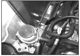
19. Secure the front heat shield bracket to the front air box location with the provided hardware.
