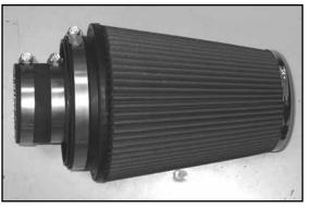
31. Install silicone hose (#08630) onto the air filter adapter and secure with the provided hose clamp.
