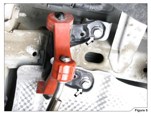
**!** WARNING: make sure, that you support the stock muffler during this process or you could injure yourself or damage the vehicle!
