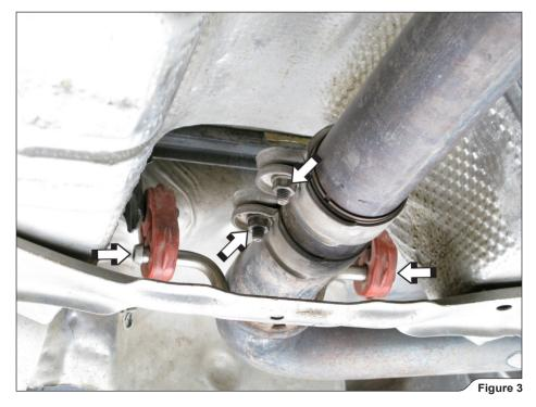
! WARNING: make sure, that you support the stock link-pipe during this process or you could injure yourself or damage the vehicle!
