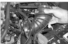
Loosen the hose clamp at the throttle body, then remove the stock intake tube as shown.
