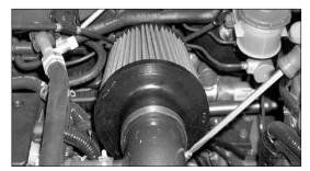
23. Install the K&N® air filter onto the K&N® intake tube, then, secure with the provided hose clamp as shown.
