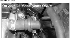
14. On '05-'06 models, remove the stock crank case vent hose as shown.
