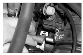
5. Disconnect the IA bypass control thermal valve vent hose from the stock intake tube as shown.
