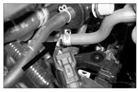
12. Remove the stock IA bypass control thermal valve vent hose as shown.
