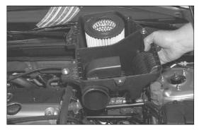
8. Remove the one hex nut and loosen the two hex bolts that secure the lower air cleaner assembly, then remove the assembly as shown.
