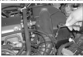
6. Loosen the hose clamp at the air cleaner assembly as shown.
