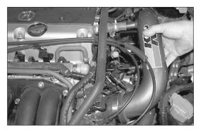
17. Slide the K&N® intake tube into the silicone hose on the throttle body, then line up the bracket on the tube with the original air cleaner mounting point as shown.
