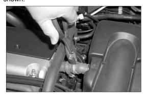
3. Depress and slide the hose clamp off the crank case vent connection at the air cleaner assembly as shown.
