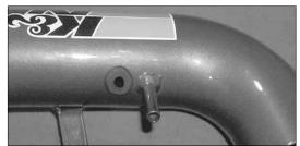
16. Install the provided grommet into the hole on the  $K\&N^{\circ}$  intake tube as shown.
