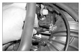
4. Depress the hose clamp at the air temperature sensor, then remove the air temperature sensor from the stock intake tube as shown.
