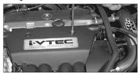
25. Reinstall the engine cover and secure with the original hex bolts as shown.
