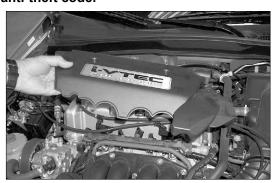
2. Loosen and remove the two bolts that secure the engine cover, then remove the engine cover as shown.
