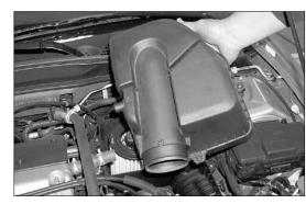
7. Loosen the five bolts that secure the upper air cleaner assembly, then remove the assembly as shown.
