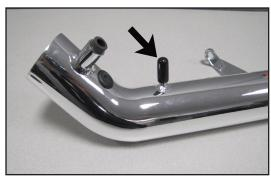
15. On models without the FIAC valve, plug the vent on the K&N® Typhoon® short ram tube with the provided cap plug.
