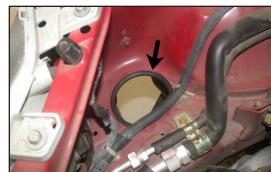
23. Install the provided edge trim onto the hole in the inner fender as shown.
