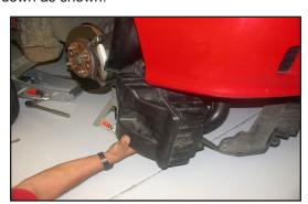
11. Remove the two bolts that secure the resonator to the inner fender, then, remove the resonator as
