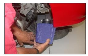
30. From underneath the vehicle install the air filter onto the cold air tube and secure using the provided hose clamp.
