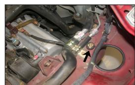
24. Insert the rubber mounted stud into the threaded hole on the inner fender as shown.
