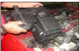
6. Pull firmly upwards to release the air cleaner from the lower grommet, then, remove the air cleaner assembly as shown.
