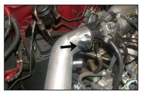
21. Insert the air temperature sensor into the grommet on the K&N® short ram tube as shown.
