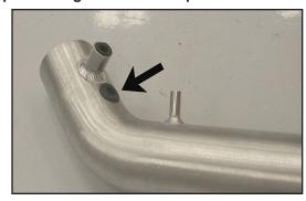
14. Install the provided grommet into the hole on the K&N® Typhoon® short ram tube as shown.
