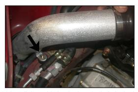
26.Install the cold air tube into the hole in the inner fender, then, line up the bracket with the rubber mounted stud as shown.
