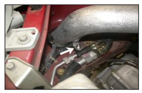
28. Secure the bracket to the rubber mounted stud using the provided hardware as shown, but do not tighten at this time.
