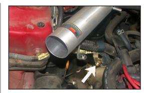
19. Slide the intake tube into the silicone hose on the throttle body, then, slide the "Z" bracket in between the starter bracket and the wire harness bracket, then, secure it using the stock bolt removed in step 16.
