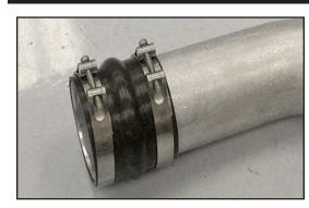
25. Install the silicone hose and hose clamps onto the K&N® cold air tube as shown, but do not tighten at this time.
