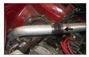
27. Slide the silicone hose over the K&N® Typhoon® short ram tube as shown, but do not tighten at this time.
