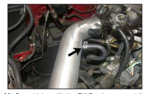
22. On vehicles with the FIAC valve connect the hose to the vent on the K&N® Typhoon® short ram tube as shown.
