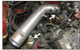
17.On automatic transmission vehicles (manual transmission vehicles go to the step 18) slide the tube into the silicone hose, then, slide the tube bracket in between the starter bracket and the wire harness bracket, then, secure it using the stock bolt from step 16.
