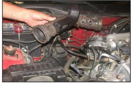
4. Loosen the hose clamp at the throttle body, then, remove the stock intake hose from the vehicle as shown.
