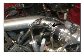
20. Insert the crankcase vent hard line into the vent on the K&N® Typhoon® short ram tube as shown.
