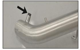
13. Install the provided silicone hose into the vent on the K&N® Typhoon® short ram tube as shown, mark, the excess hose and trim to fit.
