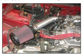
35. This K&N® Typhoon® kit has been designed to be used in two different configurations. In the case of inclement weather, the cold air tube can be removed and the air filter can be clamped onto the intake tube located in the engine compartment to avoid the possibility of ingesting water into the
