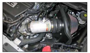
26. Install the K&N® intake tube assembly into the silicone hump hose and then into the throttle body's silicone hose. Align the tube and then secure with the provided hose clamps.
