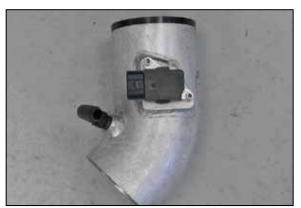
25. Install the mass air sensor into the K&N® intake tube and secure with the provided hardware.
