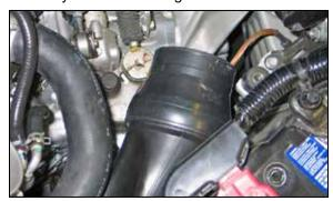
16. Install the provided silicone hose (08637) onto the fresh air intake tube as shown; secure with the provided hose clamp.
