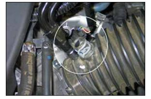
3. Release the spring clamp securing the crank case vent tube into the intake tube and then remove the crank case vent tube from the intake tube.
