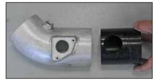
22. Install the venturi into the K&N<sup>®</sup> intake tube as shown.
