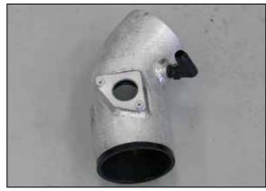
23. Install the provided 90° vent fitting into the K&N® intake tube as shown.
