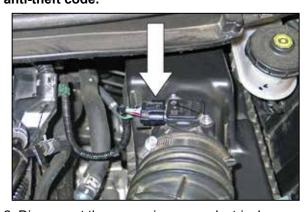
2. Disconnect the mass air sensor electrical connection and unhook the wiring harness from the upper air box.
