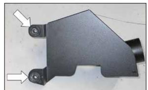
12. Install the mounting grommets from the previous step into the heat shield as shown.
