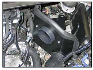
17. Install the heat shield assembly into the vehicle so the mounting grommets attach to the mounting studs, the fresh air tube aligns with the silicone hose, and the silicone hose aligns with the tube in the heat shield. Secure the heat shield with the provided hardware and hose clamp.
