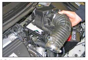
5. Release the two clips securing the upper air box to the lower air box and then remove the upper air box and intake tube assembly.
