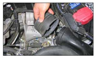
8. Remove the fresh air tube coupler as shown. NOTE: K&N Engineering, Inc., recommends that customers do not discard factory air intake.
