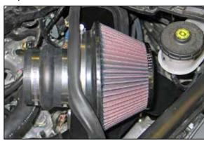
20. Install the  $K\&N^{\odot}$  air filter and secure with the provided hose clamp.
