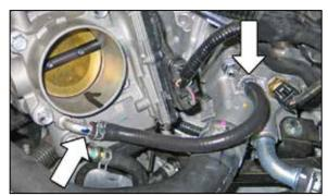
10. Be sure the engine is cool, then disconnect the coolant by-pass hoses from the engine and intake manifold. Install the provided coolant by-pass hose and secure with the factory spring clamps.
