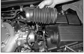
4. Loosen the hose clamp at the throttle body, then, remove the stock intake tube as shown.
