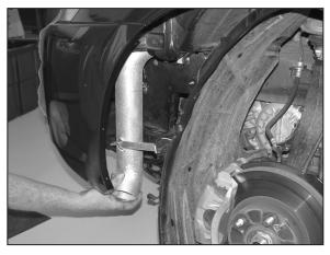
34. Slide the K&N® cold air tube into the vehicle from underneath the vehicle as shown.
