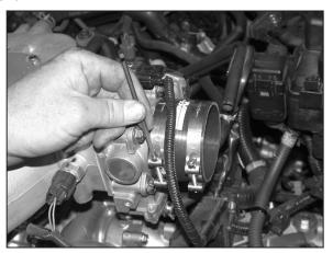
25. Install the silicone hose and hose clamps and tighten the hose clamp on the throttle body.
