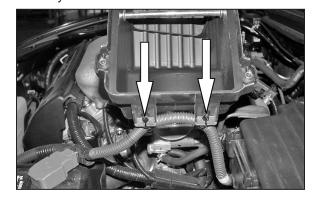
6. Rotate the upper air cleaner assembly up then using a pair of pliers unclip the wire harness and remove the upper air cleaner assembly as shown.
