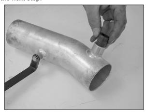
28. Slide the provided silicone hose into the vent on the K&N\$ short ram tube.
