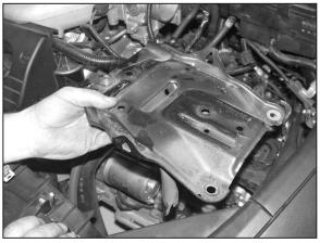
21. Remove the battery tray as shown.
