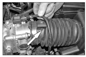
3. Unclip the wire harness from the stock intake tube as shown.
