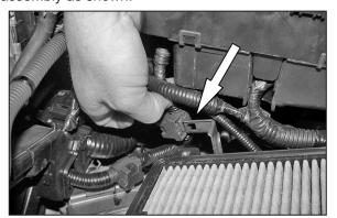
8. Using a pair of pliers unclip the wire harness from the bracket on the side of the lower air cleaner assembly as shown.
