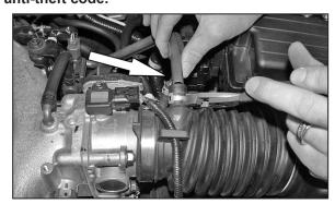
2. Depress the stock hose clamps, then, remove the crank case vent hard line from the stock intake tube as shown.
