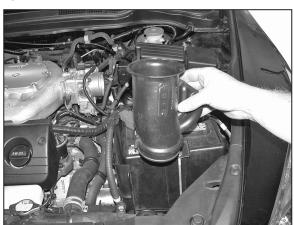
16. Remove the air inlet duct as shown.
