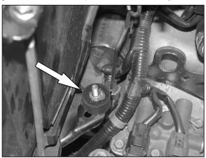
26. Install the rubber mounted stud into the original air cleaner mounting hole located directly behind the battery as shown.
