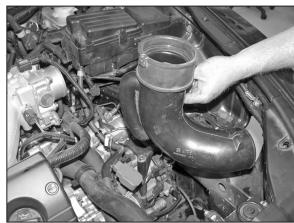
23. Remove the air inlet duct as shown.
