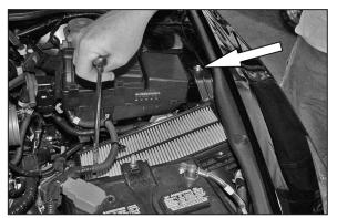
7. Loosen the two bolts on the lower air cleaner assembly as shown.
