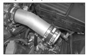
32. Slide the silicone hose and hose clamps onto the K&N® short ram tube as shown.
