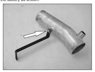
27. Secure the provided "Z" bracket to the K&N® short ram tube using the provided hardware as shown.
