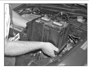
19. Remove the battery and the plastic cover as shown.
