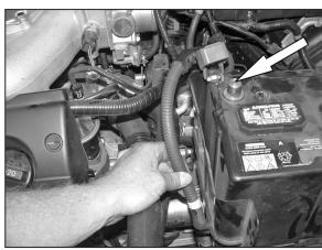
18. Disconnect the positive battery cable and unclip the cable from the side of the plastic battery cover.
