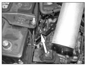
31. Secure the "Z" bracket to the rubber mounted stud using the provided hardware as shown, but do not tighten completely as this time.
