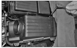
5. Loosen the four bolts on the upper air cleaner assembly.
