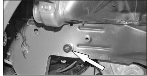
33. Install the rubber mounted stud into the original resonator mounting hole from step 13.
