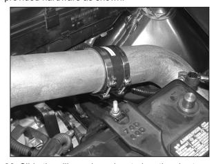
36. Slide the silicone hose located on the short ram tube onto the cold air tube as shown.
