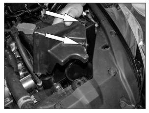
15. Located in front of battery, release the two plastic rivets, then, remove the plastic valance as shown.
