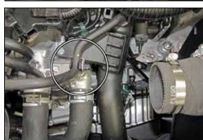
14. Remove the bypass hose retaining clip shown and flip it to the other side of the bracket and reinstall, then reinstall the bypass hose into the clip.
