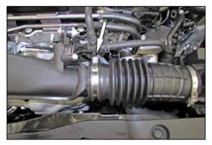
3. Loosen the hose clamp that secures the intake hose to the turbo inlet.
