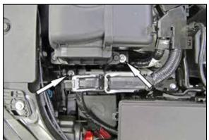
4. Remove the two bolts that secure the factory air filter housing to the inner fender and then remove the complete intake assembly from the vehicle.
