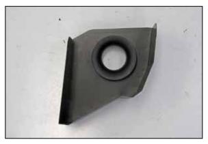
5. Install the K&N® air filter adapter into the heat shield and secure with the provided hardware.
