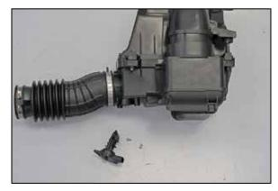
12. Remove the mass air sensor from the factory air filter housing.
