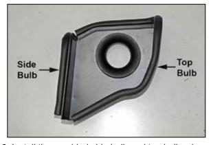
6. Install the provided side bulb and top bulb edge trim onto the heat shield as shown.
