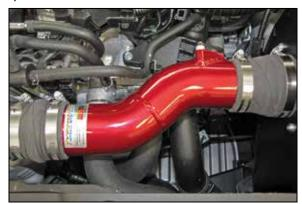
15. Install the K&N® intake tube into the hump coupler and then into the step coupler. Adjust the tube for best fit and then secure with the provided hose clamps. Reconnect the mass air sensor electrical connection.
