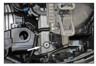
7. Thread the provided rubber mounted stud into the factory air filter housing location shown.
