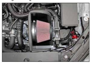
9. Flex the heat shield inward and install the K&N® air filter onto the filter adapter and secure with the provided hose clamp.
