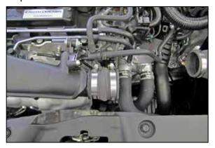
11. Install the provided hump coupler (084018) onto the turbo inlet and secure with the provided hose clamp.
