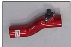
13. Install the mass air sensor into the K&N® intake tube and secure using the provided hardware.
