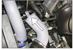
28. Install the new air inlet tube into the stock air inlet duct, then, line up the bracket with the hole on the lower air cleaner assembly and secure with the provided screw as shown.
