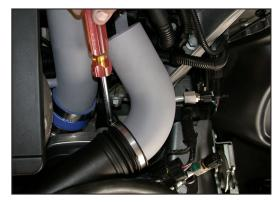
29. Tighten the provided hose clamp on the air inlet duct as shown.
