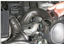
8. Remove the air cleaner inlet duct as shown.
