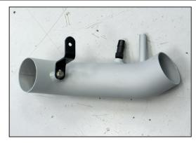
20. Secure the provided "Z" bracket onto the threaded boss on the K&N® intake tube using the provided hardware as shown.
