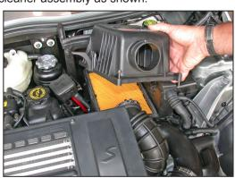
6. Slide the upper air cleaner assembly backwards, then, pull upward to remove the upper air cleaner assembly as shown.
