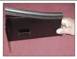
15. Install the provided edge trim onto the K&N<sup>®</sup> heat shield as shown.
