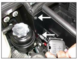
17. Using the two screws from step 14, secure the heat shield to the bulkhead as shown.
