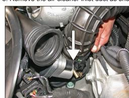
9. Remove the throttle body electrical connection as shown.
