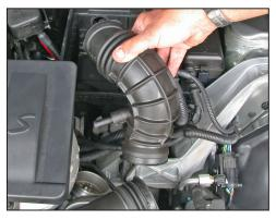
12. Remove the stock intake tube as shown.
