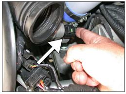
27. Reconnect the throttle body electrical connection as shown.
