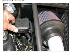
26. Slide the battery terminal onto the locating tab on the heat shield as shown.
