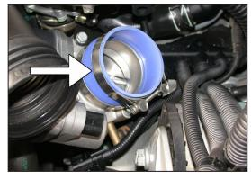
22. Install the hose clamp onto the silicone hose as shown.
