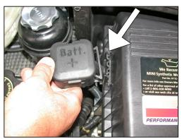
4. Pull upward to remove the battery terminal from the side of the air cleaner as shown.
