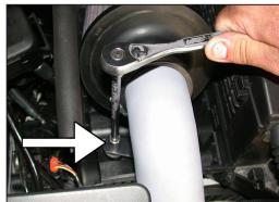
24. Using the provided hardware secure the "Z" bracket to the rubber mounted stud as shown.
