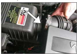
3. Pull the stock intake tube off the air cleaner as
