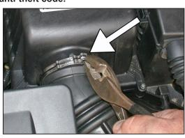
2. Using a pair of dikes or pliers unclip the stock hose clamp at the air cleaner as shown.
