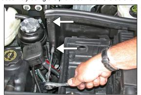
14. Remove the two stock bolts on the bulkhead as shown.
