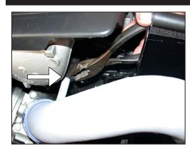
25. Reconnect the stock crank case vent hose to the vent on the intake tube as shown.
