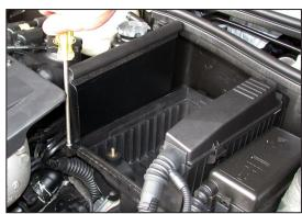
18. Tighten all hardware on the heat shield as shown.
