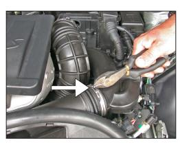
7. Using a pair of dikes or pliers unclip the hose clamp on the air inlet duct as shown.
