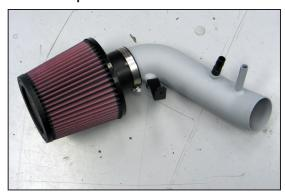
21. Install the K&N® air filter onto the K&N® intake tube and tighten with the provided hose clamp as shown.
