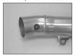
17. Install the grommet provided into the K&N<sup>®</sup> intake tube as shown.
