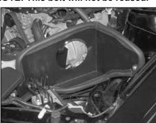
14. Install the heat shield and secure with the provided hardware as shown.
