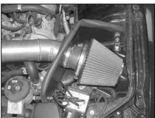
26. Install the air filter assembly onto the K&N® intake tube as shown and secure with the provided hose clamp.
