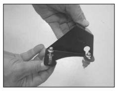
8. Install the valve cover bolts removed in step #7 into the tube mounting bracket as shown passing through the key hole portion and then slide the bolts to the end of the slots.
