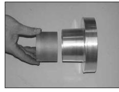
23. Place the Hydrocarbon trap into the filter adapter as shown.
