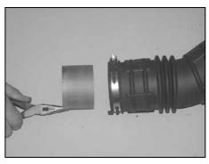
22. This step only applies to 2005 models equipped with an air box part number of 4R33-9C662-BJ or 4R33-9C662-CF, use a pair of needle nose pliers and remove the Hydrocarbon trap from the stock intake tube as shown.
