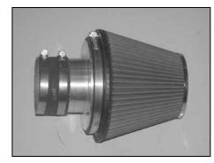
25. Install the air filter onto the filter adapter and secure with the provided hose clamp as shown.
