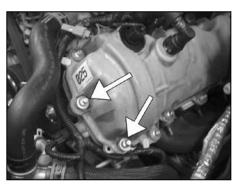
7. Remove the two valve cover bolts shown. **NOTE: These bolts will be reused.**
