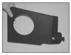
11. Install the "L" bracket (07158) onto the front of the heat shield as shown with the provided hardware.
