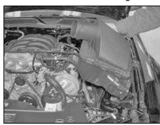
6. Remove the air box assembly as shown. NOTE: K&N recommends customers do not discard their factory air intake.
