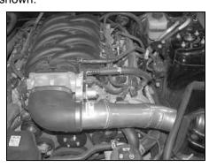
19. Install the K&N® intake tube into the silicone hose at the throttle body and onto the mounting bracket installed in step #9, then secure with provided hose clamp and 6mm bolt.
