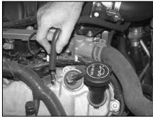
21. Install the crank case vent hose mender into the grommet installed in the K&N® intake tube and then onto the valve cover as shown.
