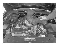
4. Loosen the hose clamps, which secure the intake tube to the throttle body and air box, then remove the intake tube as shown.
