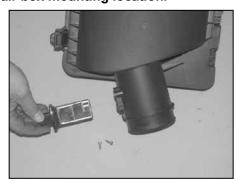
15. Remove the mass air sensor from the factory air box with the T20 "TORX" wrench provided.
