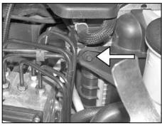
13. Remove the radiator fan shroud mounting bolt shown
