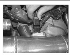
27. Reconnect the mass air sensor electrical connection as shown.
