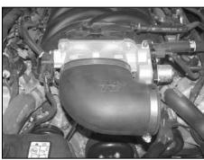
18. Install the silicone hose (084094) onto the throttle body with the provided hose clamp as shown.
