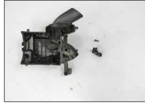
19. Remove the inlet air temperature sensor from the factory air filter housing.
