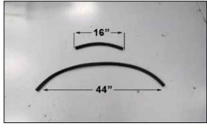
14. Cut the provided edge trim into two sections, one section will be 16" long and the other section will be 44" long.
