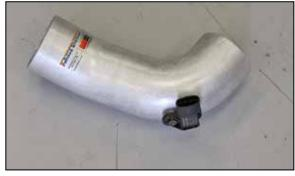
20. Install the inlet air temperature sensor into the grommet installed into the K&N<sup>®</sup> intake tube.
