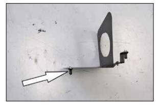
12. Install the remaining mounting stud onto the heat shield as shown using the provided hardware.
