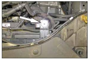
16. Place the provided rubber and fender washer onto the front air filter housing mount as shown
