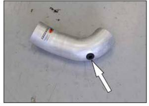
18. Install the provided grommet into the K&N<sup>®</sup> intake tube as shown.
