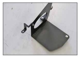
13. Install the provided bracket (064334) onto the heat shield as shown.
