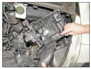
7. Lift up the lower air filter housing to dislodge it from the mounting grommets then rotate the housing up and remove it from the vehicle. Remove the factory intake tube at this time. **NOTE: K&N Engineering, Inc., recommends that customers do not discard factory air intake.**
