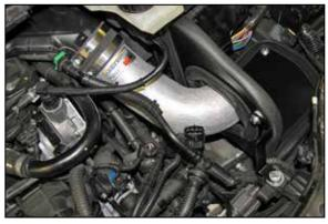
21. Install the K&N<sup>®</sup> intake tube through the heat shield and then into the coupling hose and secure with the provided hose clamp.
