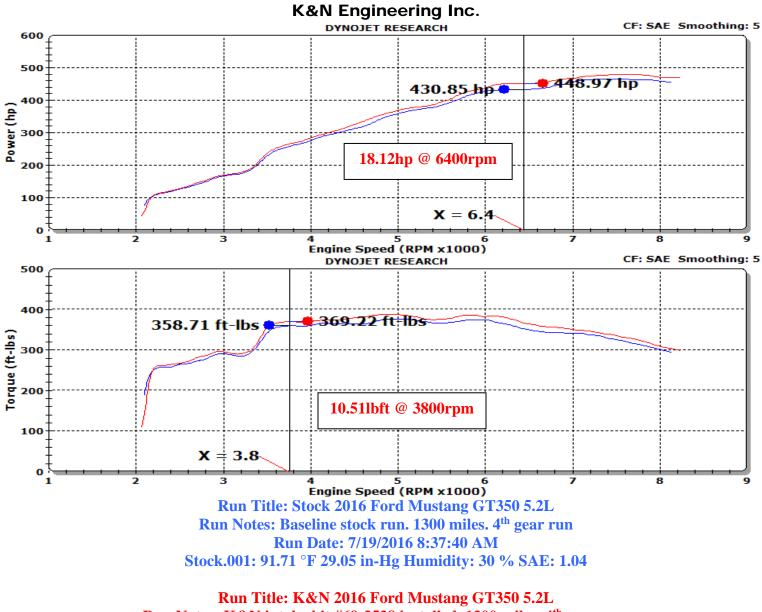
Run Notes: K&N intake kit #69-3538 installed. 1300 miles. 4<sup>th</sup> gear run. Run Date: 7/19/2016 9:50:10 AM K&N.002: 92.24 °F 29.05 in-Hg Humidity: 29 % SAE: 1.04
