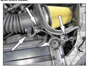
2. Disconnect the mass air sensor electrical connection and unhook the wiring harness from the mounting studs.
