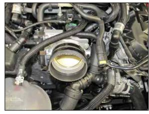
17. Install the provided coupler (08618) onto the throttle body and secure with the provided hose clamp.
