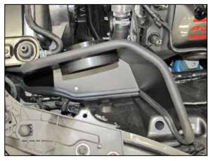
14. Install the heat shield onto the lower mounting bracket and secure it to the mounting bracket only with the provided hardware.
