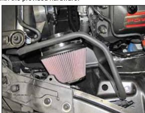
15. Lean the heat shield in enough to install the K&N® air filter onto the adapter and secure the filter with the provided hose clamp. Then secure the heat shield mounting bracket to the inner fender with the provided hardware.
