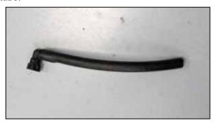
23. Install the provided 5/8 quick disconnect fitting into the provided crank case breather hose.
