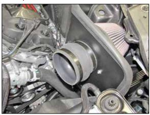
16. Install the provided hump coupler (08418) onto the filter adapter and secure with the provided hose clamp.
