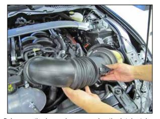
5. Loosen the hose clamp securing the intake tube to the throttle body and then remove the intake tube and filter from the vehicle.
