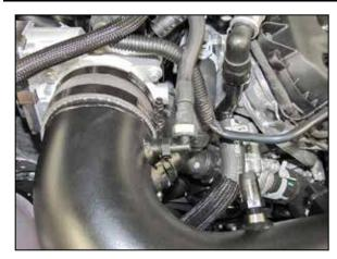
22. Connect the EVAP vent line to the quick disconnect fitting installed into the K&N® intake tube.
