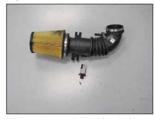
18. Remove the mass air sensor from the factory intake tube.
