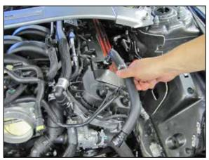
9. Remove the crank case vent hose from the valve cover.
