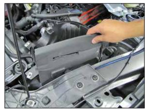
6. Remove the foam air dam from the inner fender.
