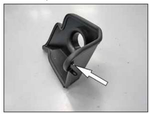
13. Install the provided heat shield bracket (064326) onto the heat shield and secure with the provided hardware.
