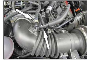
4. Disconnect the crank case and evap vent lines from the intake tube.
