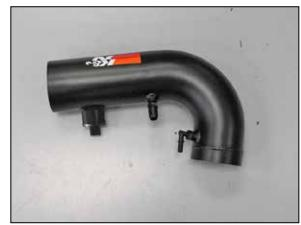
20. Install the two vent fittings into the  $K\&N^{\otimes}$  intake tube as shown.
