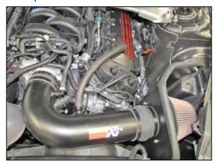
24. Install the crank case breather hose onto the valve cover port using the quick disconnect fitting and then install the open end onto the fitting installed into the K&N® intake tube.
