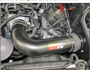
21. Install the K&N® intake tube into the coupler at the filter adapter and then into the coupler at the throttle body, adjust the tube for best fit and then secure with the provided hose clamps.
