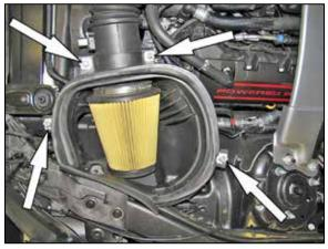
3. Remove the four mounting studs that secure the upper heat shield and then remove the upper heat shield.
