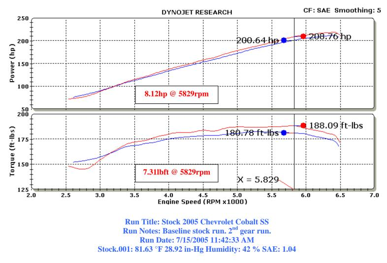
Run Title: K&N 2005 Chevrolet Cobalt SS Run Notes: K&N intake kit #69-4516 installed. 2<sup>nd</sup> gear run Run Date: 7/15/2005 11:46:21 AM K&N.002: 89.34 °F 28.90 in-Hg Humidity: 25 % SAE: 1.04
