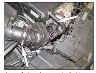
4. Loosen the hose clamps securing the intake tube to the turbo inlet and mass air sensor, and then remove the factory intake tube from the vehicle.
