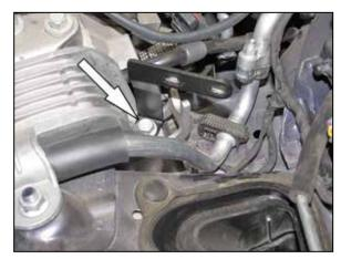
7. Install the heat shield mounting bracket (083149) onto the engine mount and secure it with the bolt removed in the previous step.
