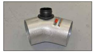
13. Install the provided quick disconnect fitting into the grommet installed into the K&N® intake tube.
