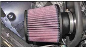
18. Install the K&N® air filter and secure it with the provided hose clamp.
