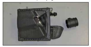
15. Loosen the hose clamp and remove the mass air sensor from the factory air filter housing
