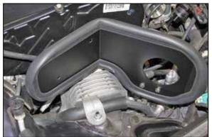
9. Install the heat shield onto the mounting bracket and secure with the provided hardware and spacers, the spacers are to be placed between the bracket and heat shield.
