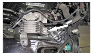
6. Remove the motor mount bolt show.
