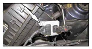
5. Lift up the air filter assembly to gain access to the electrical box attached to the air filter housing. Remove the two bolts that secure the electrical box and separate it from the air filter housing and then remove the air filter assembly from the vehicle.
