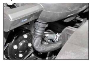
4. Release the sound tube quick disconnect fitting and disconnect the sound tube from the factory intake tube.
