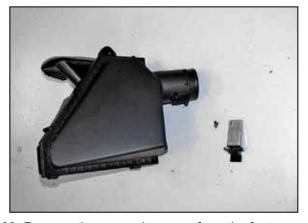
22. Remove the mass air sensor from the factory air filter housing.
