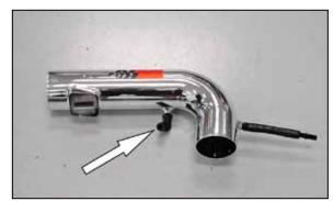
21. Install the  $90^{\circ}$  crank case vent fitting into the K&N® intake tube as shown.
