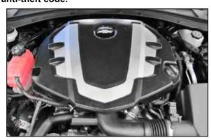
2. Remove the bolt that secures the decorative engine cover, remove the oil cap and then remove the decorative engine cover. Reinstall the oil cap.
