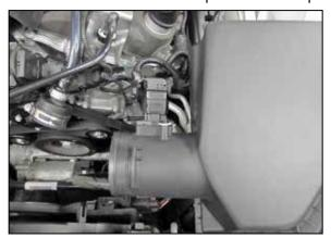
9. Disconnect the mass air sensor electrical connection.
