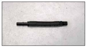
19. Assemble the provided EVAP fittings and hose as shown.
