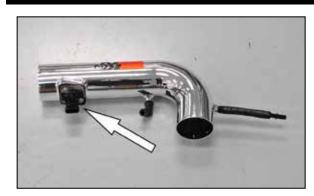
23. Install the mass air assembly into the K&N® intake tube as shown.
