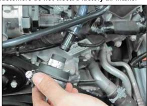
11. Remove the factory crank case vent coupler from the crank case vent tube.
