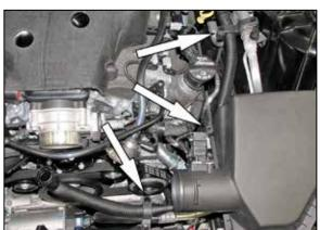
6. Release the three flexible clamps that secure the sound tube and disconnect the sound drum from the rear sound tube then remove the sound tube
