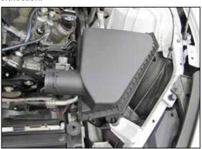
10. Lift up and remove the factory air filter housing assembly.
