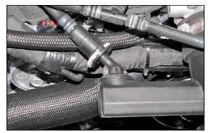
3. Release the locking tap and then disconnect the EVAP vent line quick disconnect fitting from the factory intake tube.
