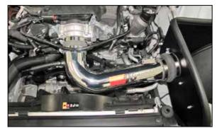
24. Install the K&N® intake tube assembly into the coupler at the filter adapter and then into the coupler on the throttle body, adjust the tube for best fit and then secure with the provided hose clamps.
