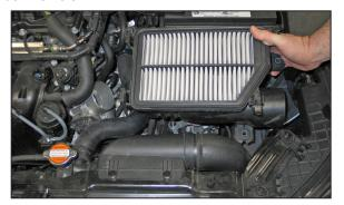
8. Remove the lower air box assembly from the vehicle.
