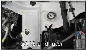
13. Install the  $\frac{1}{2}$ " rubber mounted stud into the rear/inner air box mounting box location.
