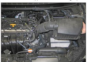
6. Remove the upper air box/ intake hose assembly from the vehicle.
