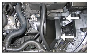
16. Install the heat shield onto the previously installed rubber mounted studs and secure with the provided hardware.
