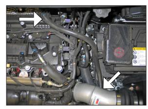
23. Install the provided crank case vent hose onto the 90° fitting in the K&N® intake tube. Attach the opposite end to the valve cover vent port.
