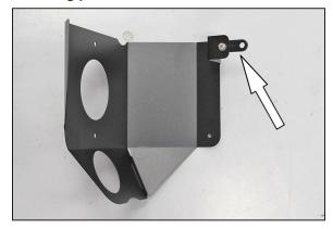
13a. On 2013 and later model vehicles, install the provided bracket (07133) onto the heat shield as shown,
