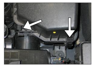
5. Release the two upper air box retaining clips.
