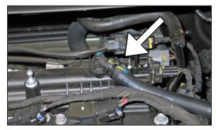
3. Release the spring clamp that secures the crank case vent hose to the valve cover port and then disconnect the crank case vent hose from the valve cover.
