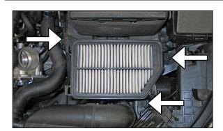
7. Remove the three bolts that secure the lower air box vehicle.
