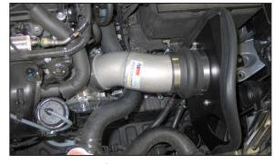
20. Install the K&N® intake tube into the silicone hump hose and then into the silicone hose attached to the throttle body. Secure with the provided hardware.
