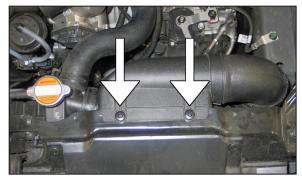
9. Push the centers of the fresh air duct retaining pins down to release the clips.
