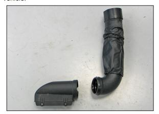
11. Remove the fresh air duct from the fresh air scoop.
