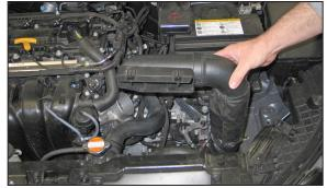
10. Remove the fresh air intake duct from the vehicle.
